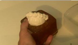
Next, pull out the master, add the wick, and pour in the wax. If the wax is above 130 F, freeze your mold first by placing it in the freezer until thoroughly chilled.
