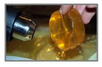
Because of the thermoplastic nature of ComposiMold, it has the advantage of being able to be patched through heating. This can provide unique molding capabilities for the creative mold maker. For example, molds can be adapted, patched, attached together, holes patched in the molds, or gaps filled or made with purpose.
